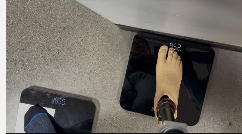
Trial 2: Left = 105lbs, Right = 95.2lbs - 9.3% loading difference
