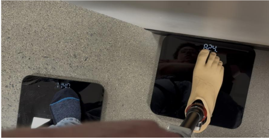
Trial 1: Left = 114lbs, Right = 82.4lbs - 27.7% loading difference
